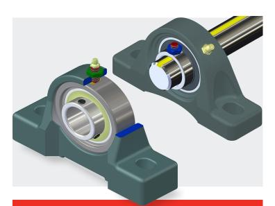
AMI offers two types of custom locking devices that are both designed to accommodate axial shaft expansion caused by high temperatures from an oven application. The two design options are specifically intended for the expansion side of an application. (Float side). \*A fixed mounted ball bearing unit should be used on the opposite side of the shaft.\* (Fixed and Float setup).
